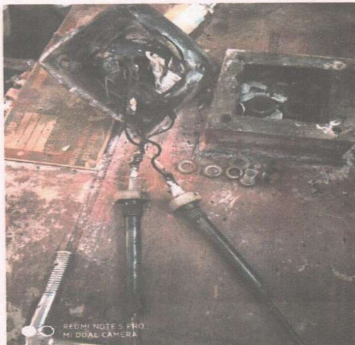
Fig. No. 4 : Badly overheated temperature sensor assembly
