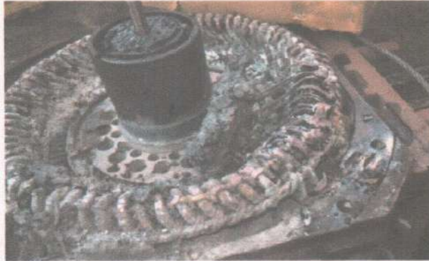
Fig 1 : DE side winding badly melted on overhang filling stator and rotor gap
