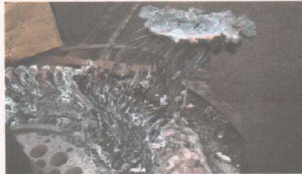
Fig No. 2&3 : Molten copper stuck on coils of winding on DE overhang
