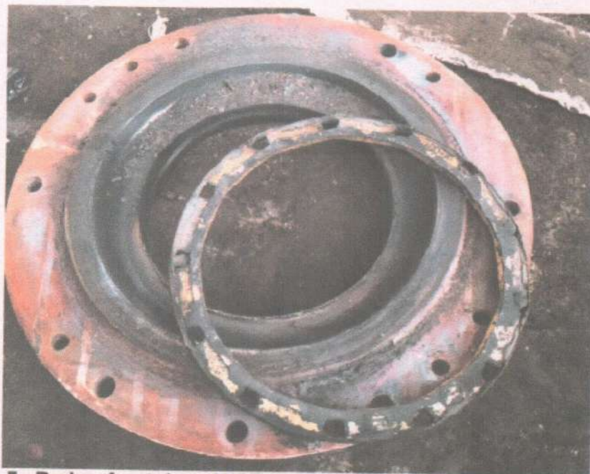
Fig. No. 7 : Broken front ring of NDE bearing brass cage and NDE grease cover
